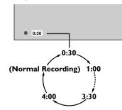
When the unit reaches the specified time, recording will stop automatically.
